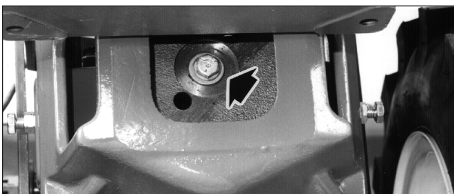
Figure 5-1: Check bolt on transmission pulley.
